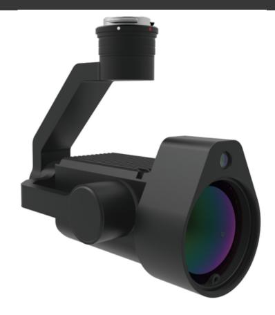
**The U10** is a lightweight, high-sensitivity gas detector based on Tunable Diode Laser Absorption Spectroscopy (TDLAS), which enables rapid identification of methane from a distance of up to 100 m, or at a concentration of 5 ppm.m.
